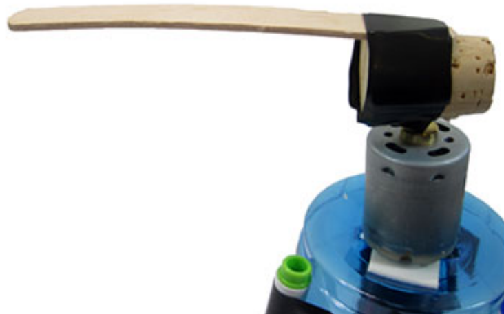
Figure 12. Securely attach the popsicle stick to the cork with electrical tape.
