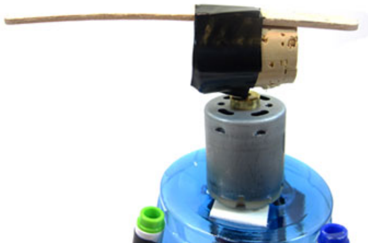
Figure 14. Popsicle stick attached to the cork so it is only partially off-center.
