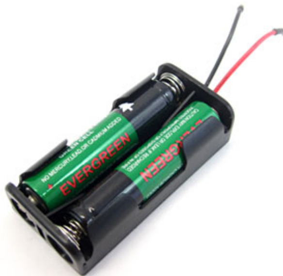
Figure 4. Put the batteries in the battery holder.
