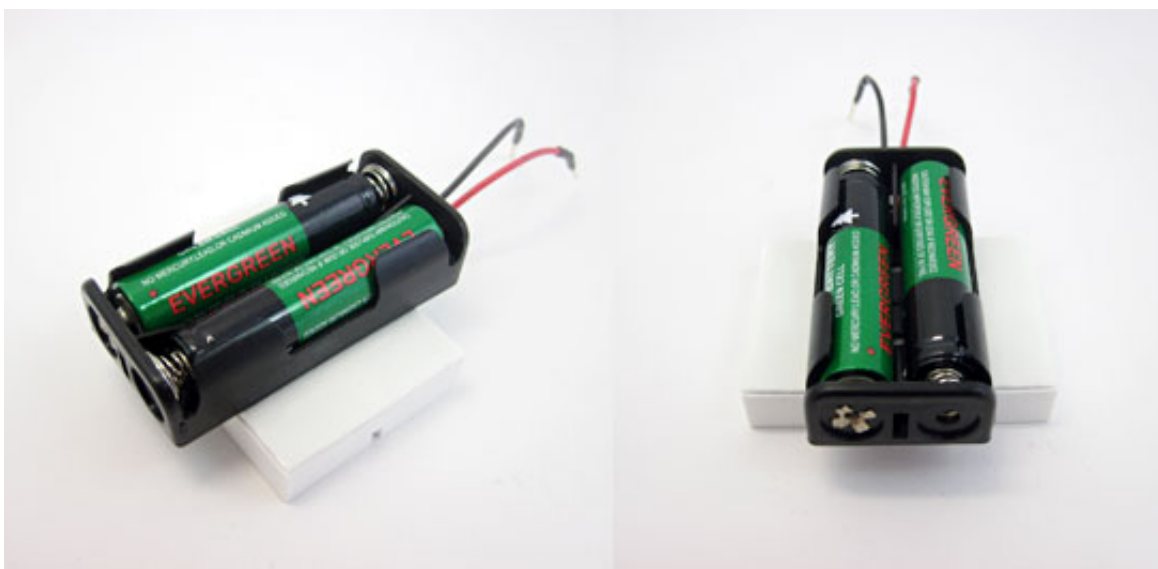
Figure 6. Mount the battery holder to the bottom of the breadboard.
