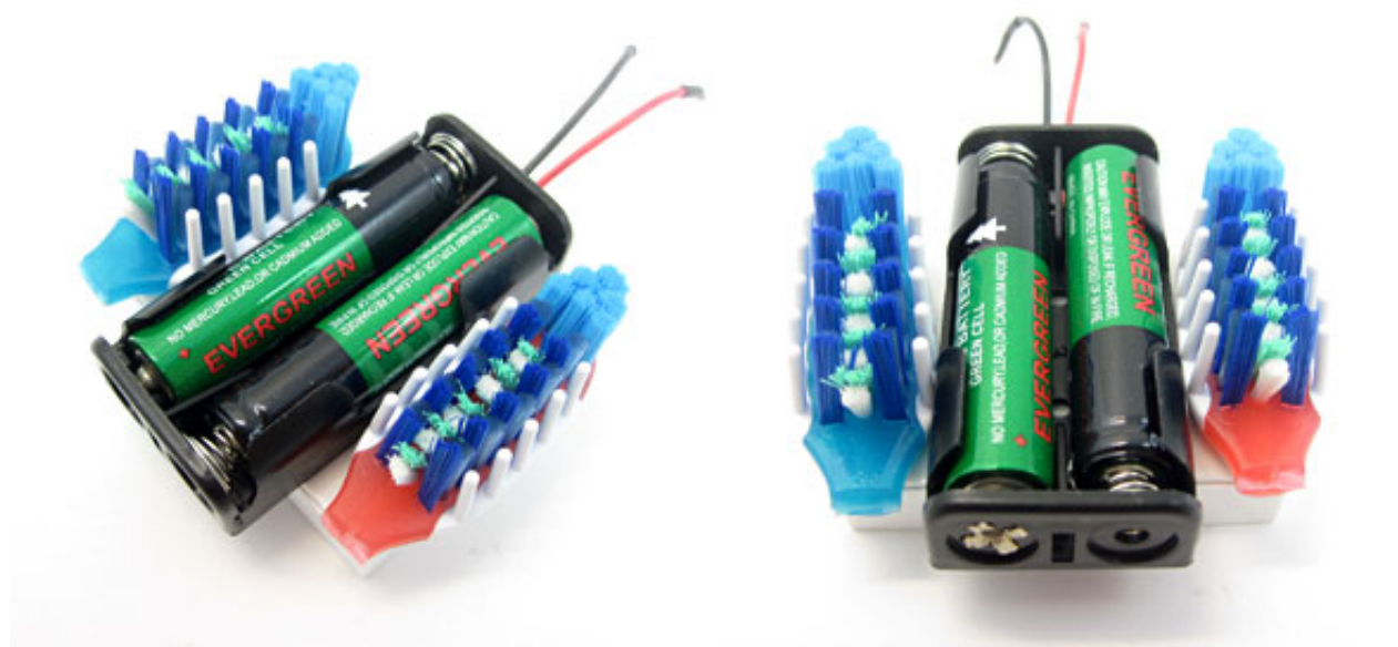
Figure 7. Mount the toothbrushes, brush-side up, next to the battery holder.
